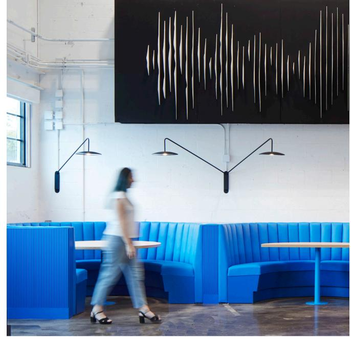
The workstation booths are outfitted with additional long-arm custom wall lights using 277V remote power and feature classic black shades. The lights provide task illumination over the worktables.
